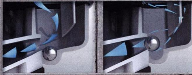
Stainless steel balls block vacuum when cups are not attached, eliminating suction of contaminants into the milk line.
